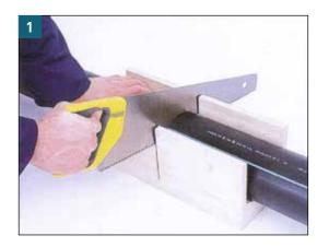
Cut the pipe squarely using special pipe cutting tools or circular or band saw. it would be better to use a sawing guide to obtain a square cut.
