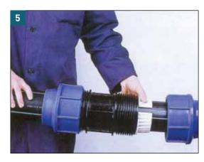
Push the white clamping ring against the body. Make sure that the clamping ring taper is in the right direction, i.e. the large part of the clamping ring must be against the body.
