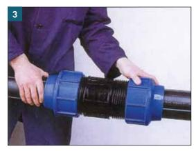
Thrust the pipe into fitting body and set the black bush and the O-ring against the body. Tighten the blue nut as far as the O-ring and the back bush go completely into the fitting body.
