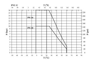
The pressure-temperature diagrams are based on a service life of 25 years and apply to water or similar media.
