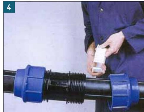
4 Unscrew the nut and put the white clamping ring onto the pipe.
