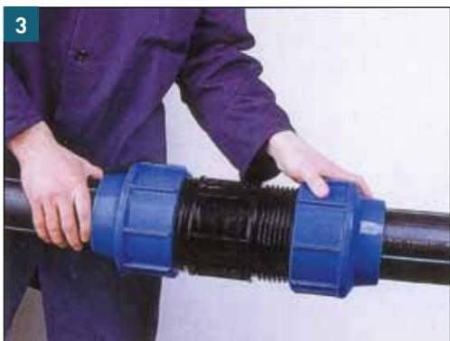
3 Thrust the pipe into fitting body and set the black bush and the O-ring against the body. Tighten the blue nut as far as the O-ring and the back bush go completely into the fitting body.
