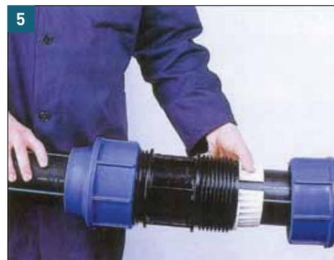
5 Push the white clamping ring against the body. Make sure that the clamping ring taper is in the right direction, i.e. the large part of the clamping ring must be against the body.
