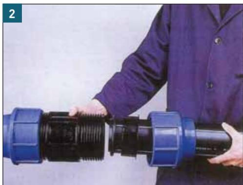
2 Disassemble all the fitting components. Make the nut, the black bush and the O-ring slide onto the pipe setting them near the pipe's end. Do not use the white clamping ring at this stage. It is helpful to lubricate the pipe's end and the O-ring with a suitable lubricant that does not affect the drinking water properties.
